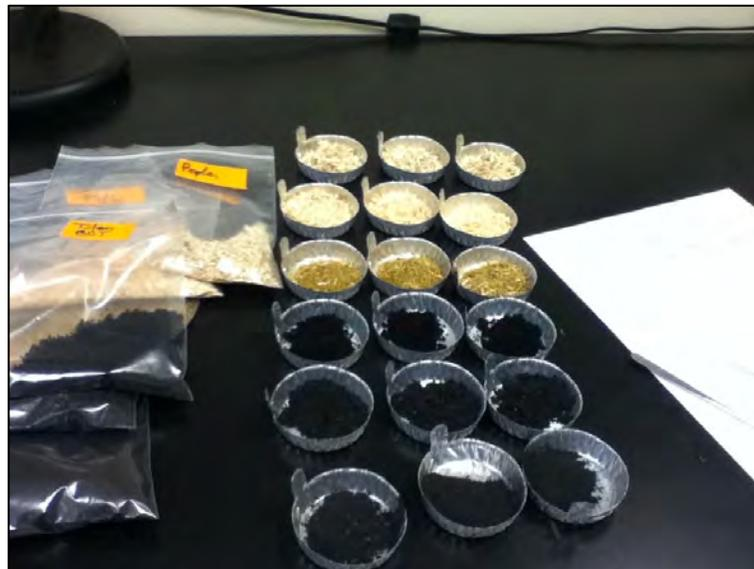
Figure 1 Biochars and wood samples tested in laboratory (grinded form)
