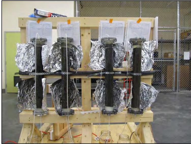
Figure 6 Bioreactors C1 to C4 (Keno Hill District conditions, 6.4 cm ID)
