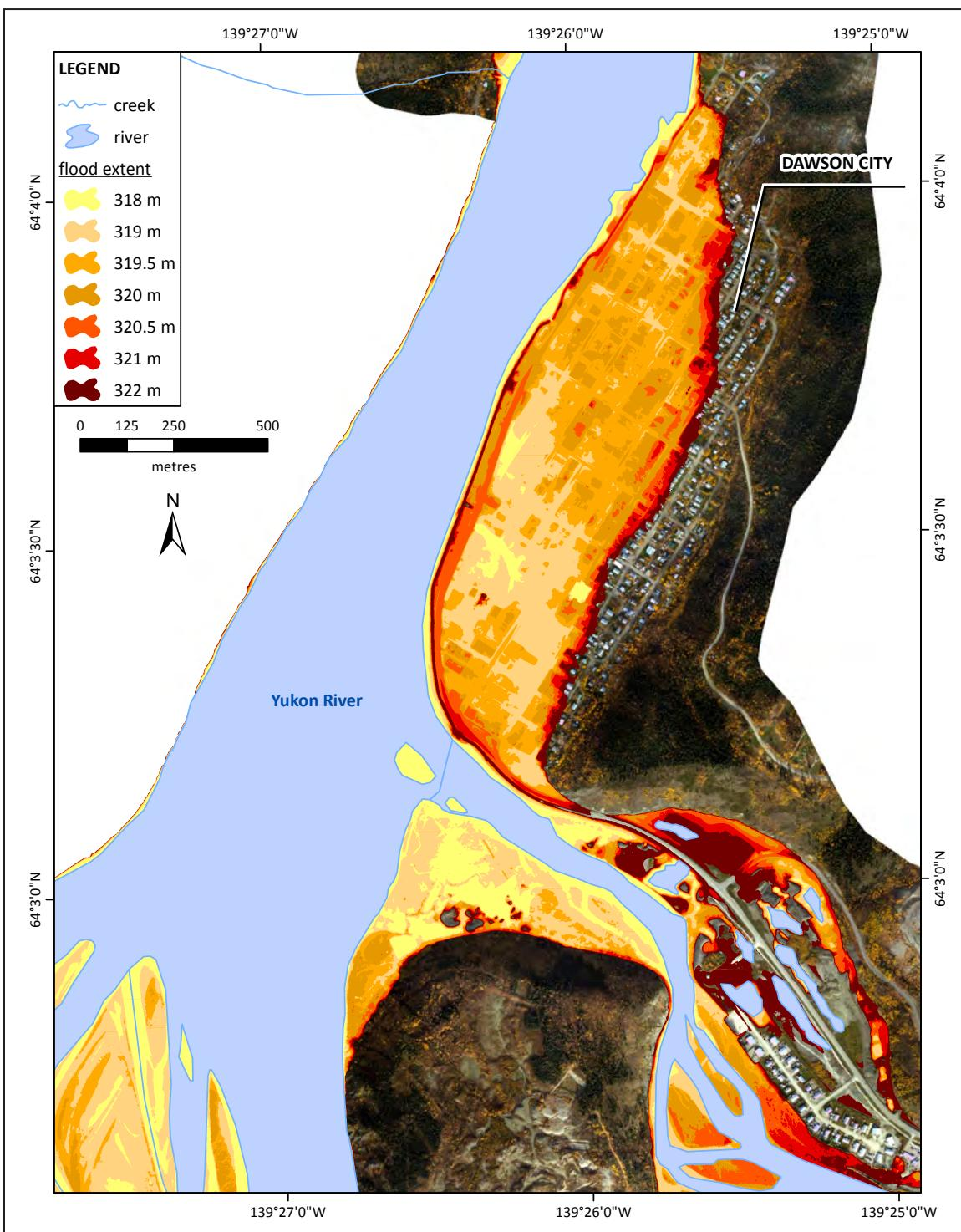
**Figure 11.** Close-up of amalgamated modelled flood extents for Dawson City illustrating Yukon River levels between 318 m and 322 m (relative to the Canadian Geodetic Datum). Note that the dike is not integrated as a barrier to flooding. Model results are based on LIDAR imagery provided by the Yukon Government. Background image source: ERSI, DigitalGlobe, GeoEye.
