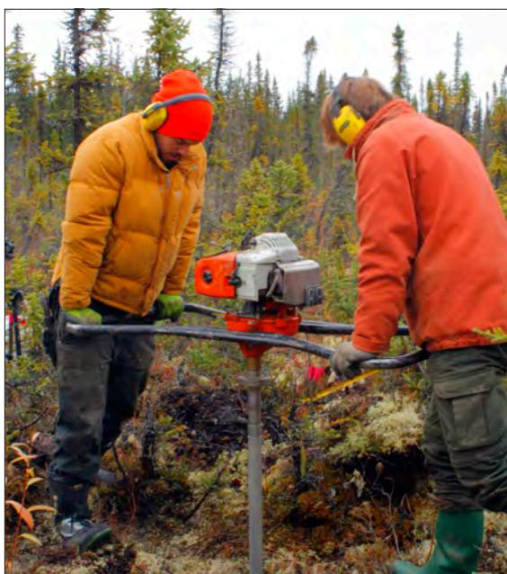
**Figure A1.** Photograph of the GÖLZ™ portable Earth-drill system used for permafrost coring.
