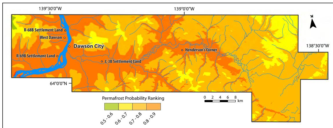
**Figure 76.** Hazard risk associated with permafrost probability in the Dawson region. Permafrost probabilities of 0.5-0.6 (equivalent to 50-60% likelihood of permafrost occurrence) are associated with lowest risk (green) while probabilities of 0.8-0.9 (equivalent to 80-90% likelihood of permafrost occurrence) are associated with highest risk (red).
