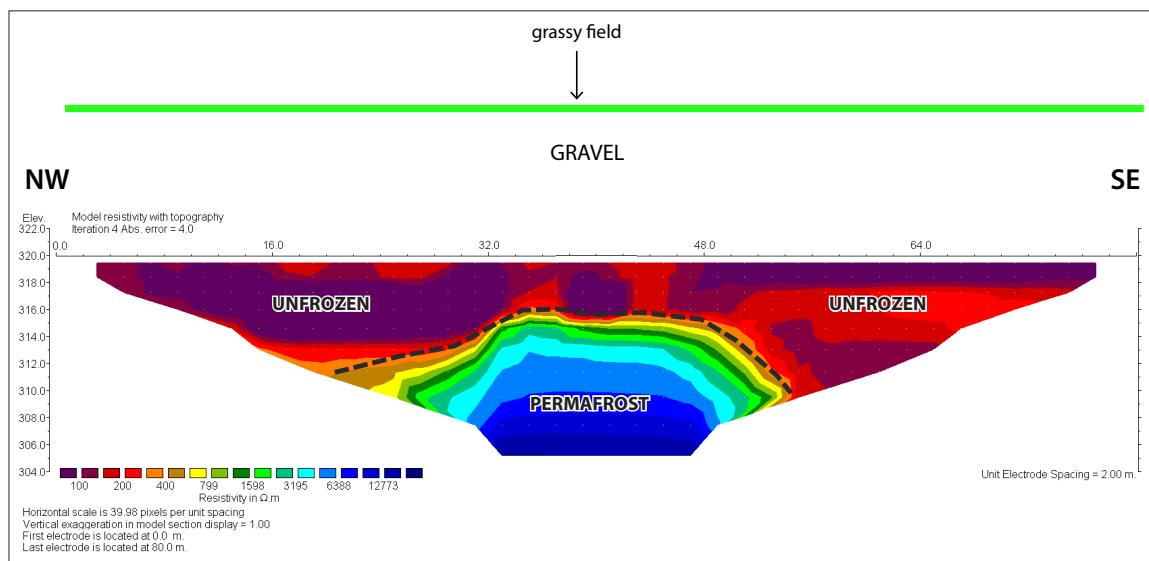
**Figure 67.** ERT profile *DC\_ERT03*, which is 80 m long and runs along the southern side of the schoolyard (see Figure 66 for location). The profile has a maximum penetration depth of ~13 m. A likely area of permafrost is outlined by a black dashed line.
