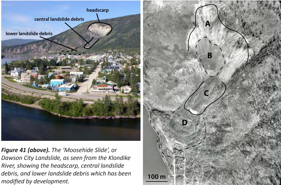
**Figure 41 (above).** The 'Moosehide Slide', or Dawson City Landslide, as seen from the Klondike River, showing the headscarp, central landslide debris, and lower landslide debris which has been modified by development.
