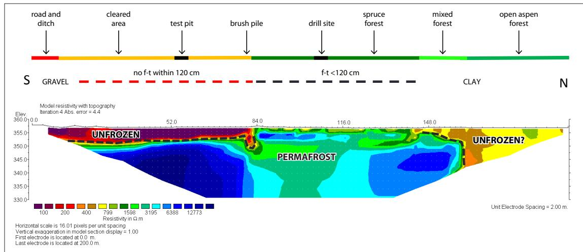
**Figure 55.** ERT profile DC\_ERT02, which is 200 m long and runs south to north across a cleared area and into forest at the C-3B case study site (see Figure 54 for location). The profile has a maximum penetration depth of ~25 m. Likely areas of permafrost are outlined by black dashed lines; f-t = frost table.
