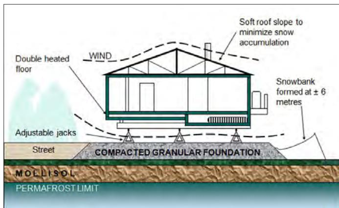
**Figure F10.** Conceptual design of a screw-jack foundation on a compact granular foundation (Gravel, 2012).
