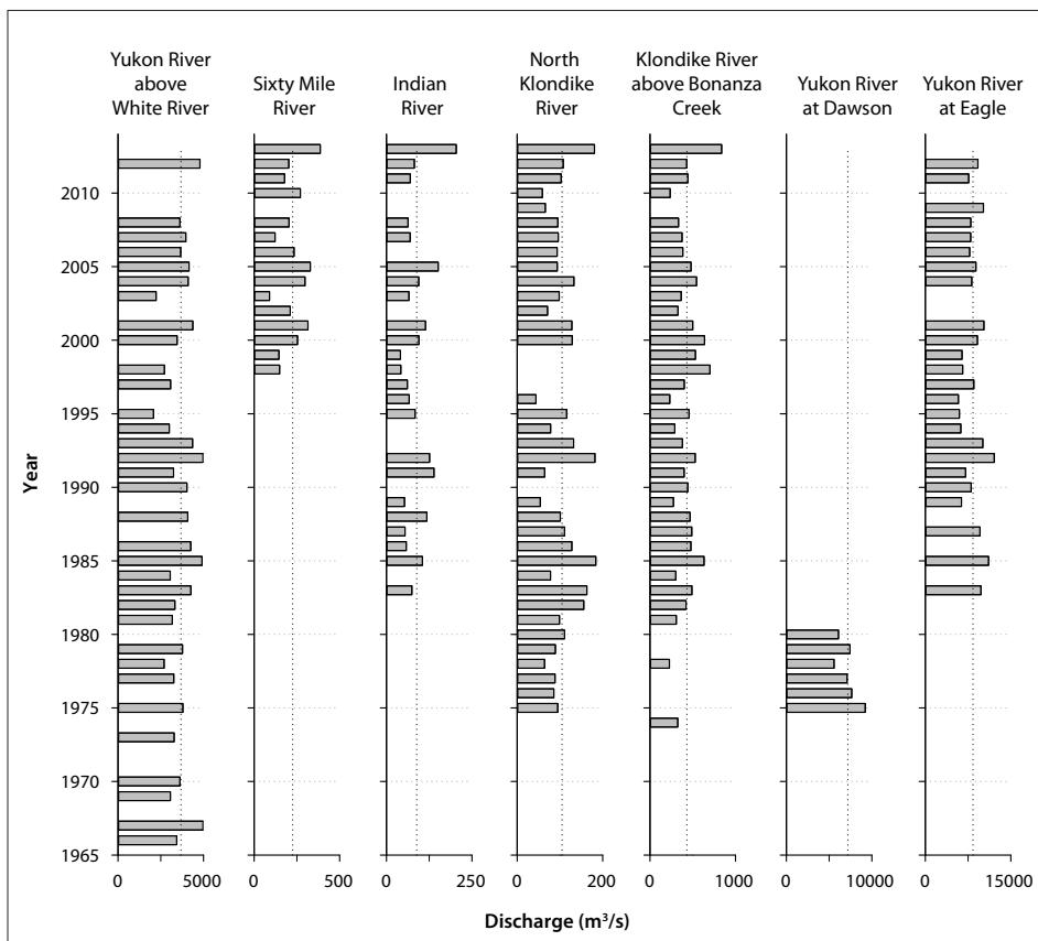
**Figure 9.** Peak discharge at WSC stations with multi-year records, arranged generally upstream (left) to downstream (right). Vertical, long-dashed lines indicate average peak discharge for each station for its period of record (Water Survey of Canada, 2015).
