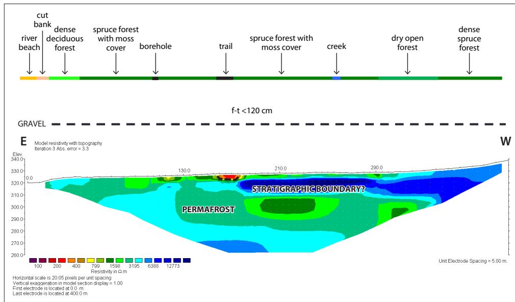
**Figure 59.** ERT profile DC\_ERT04, which is 400 m long and runs east to west from a beach along the Yukon River, into an open dwarf spruce forest (see Figure 58 for location). The profile has a maximum penetration depth of ~60 m. Likely areas of permafrost are outlined by black dashed lines; f-t = frost table.
