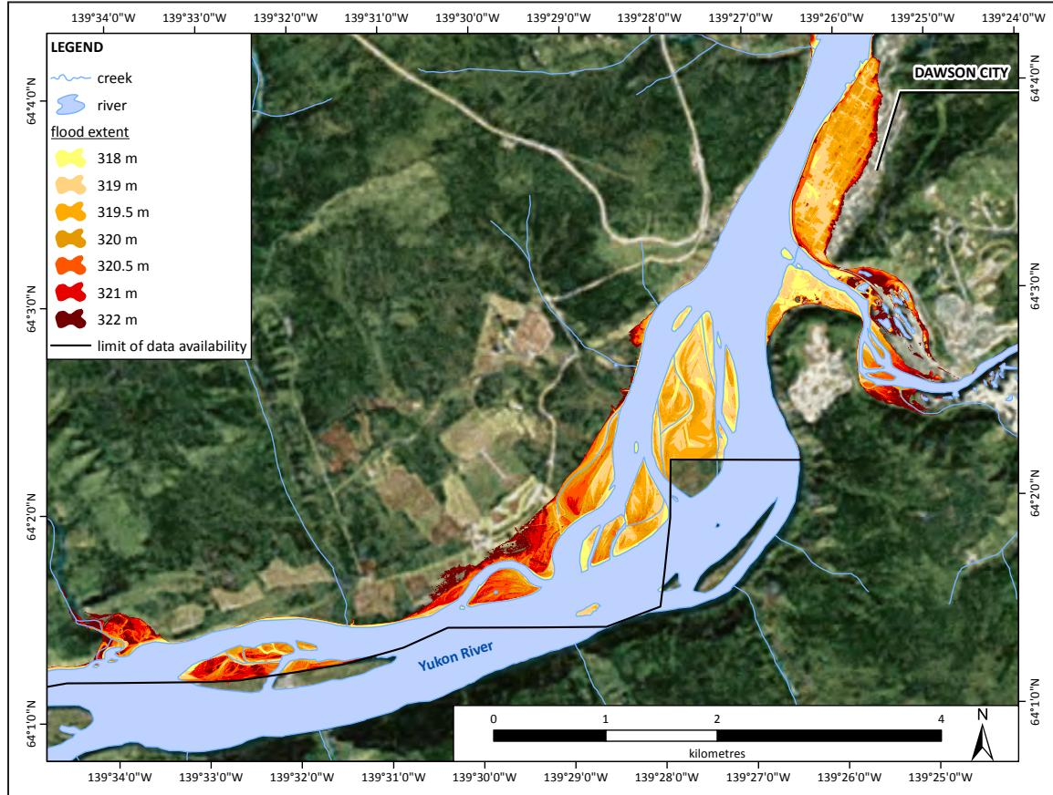
**Figure 10.** Modelled flood extents for Dawson City and surrounding area illustrating Yukon River levels between 318 m and 322 m (relative to the Canadian Geodetic Datum). Note that the dike at Dawson City is not integrated as a barrier to flooding. Model results are based on LIDAR imagery provided by the Yukon Government. Background image source: ERSI, DigitalGlobe, GeoEye.
