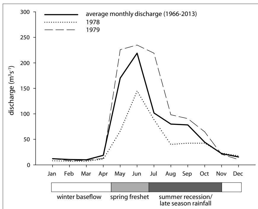
**Figure 6.** Average monthly discharge hydrograph for the Klondike River above Bonanza Creek (heavy solid line). Also shown are hydrographs for the years 1978 (dotted line) and 1979 (long-dashed line), demonstrating low and high measured peak discharge, respectively (Water Survey of Canada, 2015).
