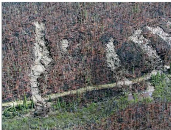
**Figure 47.** A series of active layer detachment slides generated after intense forest fire activity in 2004 blocked roads and access routes.
