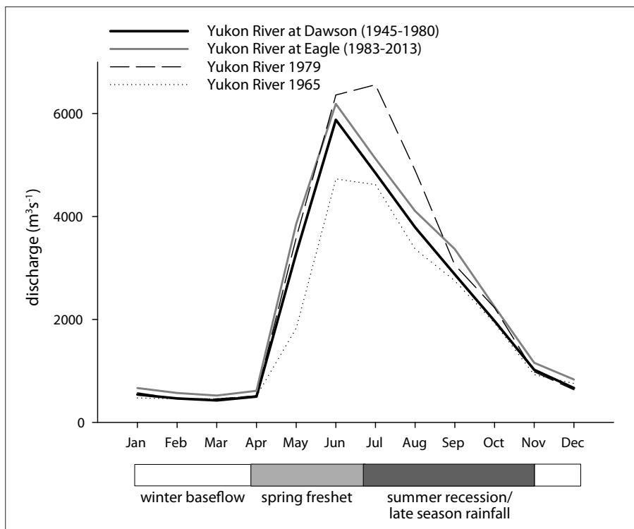
**Figure 7.** Average monthly discharge hydrograph for the Yukon River at Dawson (heavy solid line) and Eagle (heavy grey line). Also shown are hydrographs for the years 1965 (dotted line) and 1979 (long-dashed line), demonstrating low and high measured peak discharge, respectively (Water Survey of Canada, 2015).
