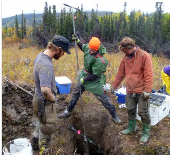
**Figure A5.** Photograph of the hand auger, used for permafrost coring.
