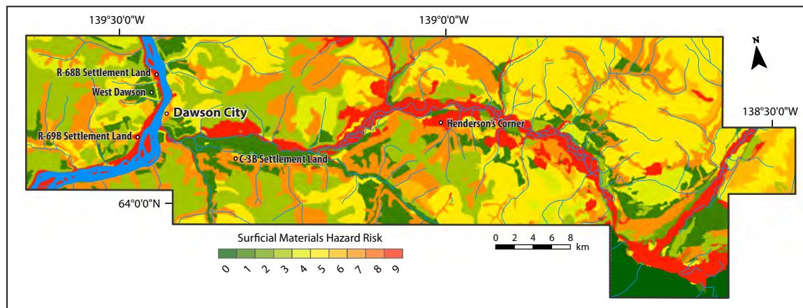
**Figure 77.** Hazard risk associated with surficial materials in the Dawson region. Stable geological units (e.g., fluvial and glaciofluvial landforms above floodplains, weathered bedrock, coarse-grained colluvium overlying bedrock) are classified as lowest risk (dark green) while geological units affected by landslides, thermokarst, ice-wedge polygons or flooding are classified as highest risk (dark red).
