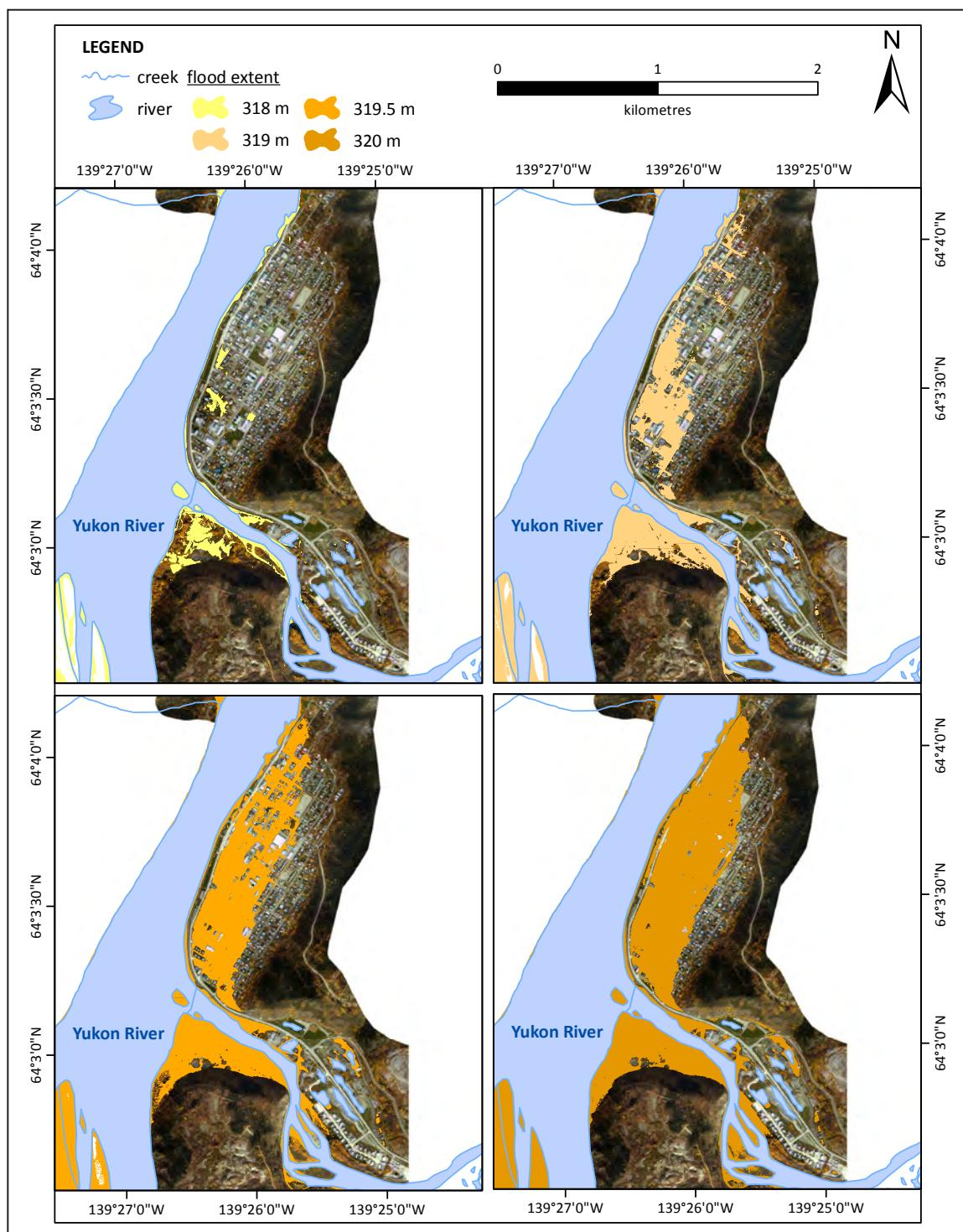
**Figure 12a.** Modelled flood extents for Dawson City depicting flood extent for individual Yukon River levels (relative to the Canadian Geodetic Datum) including river levels of 318, 319, 319.5 and 320 m. Note that the dike is not integrated as a barrier to flooding. Model results are based on LIDAR imagery provided by the Yukon Government. Background image source: ERSI, DigitalGlobe, GeoEye.
