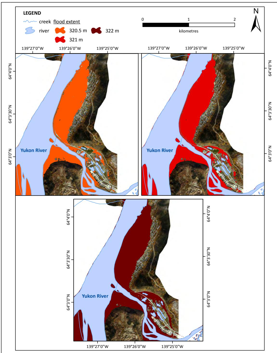
**Figure 12b.** Modelled flood extents for Dawson City depicting flood extent for individual Yukon River levels (relative to the Canadian Geodetic Datum) including river levels 320.5, 321 and 322 m. Note that the dike is not integrated as a barrier to flooding. Model results are based on LIDAR imagery provided by the Yukon Government. Background image source: ERSI, DigitalGlobe, GeoEye.
