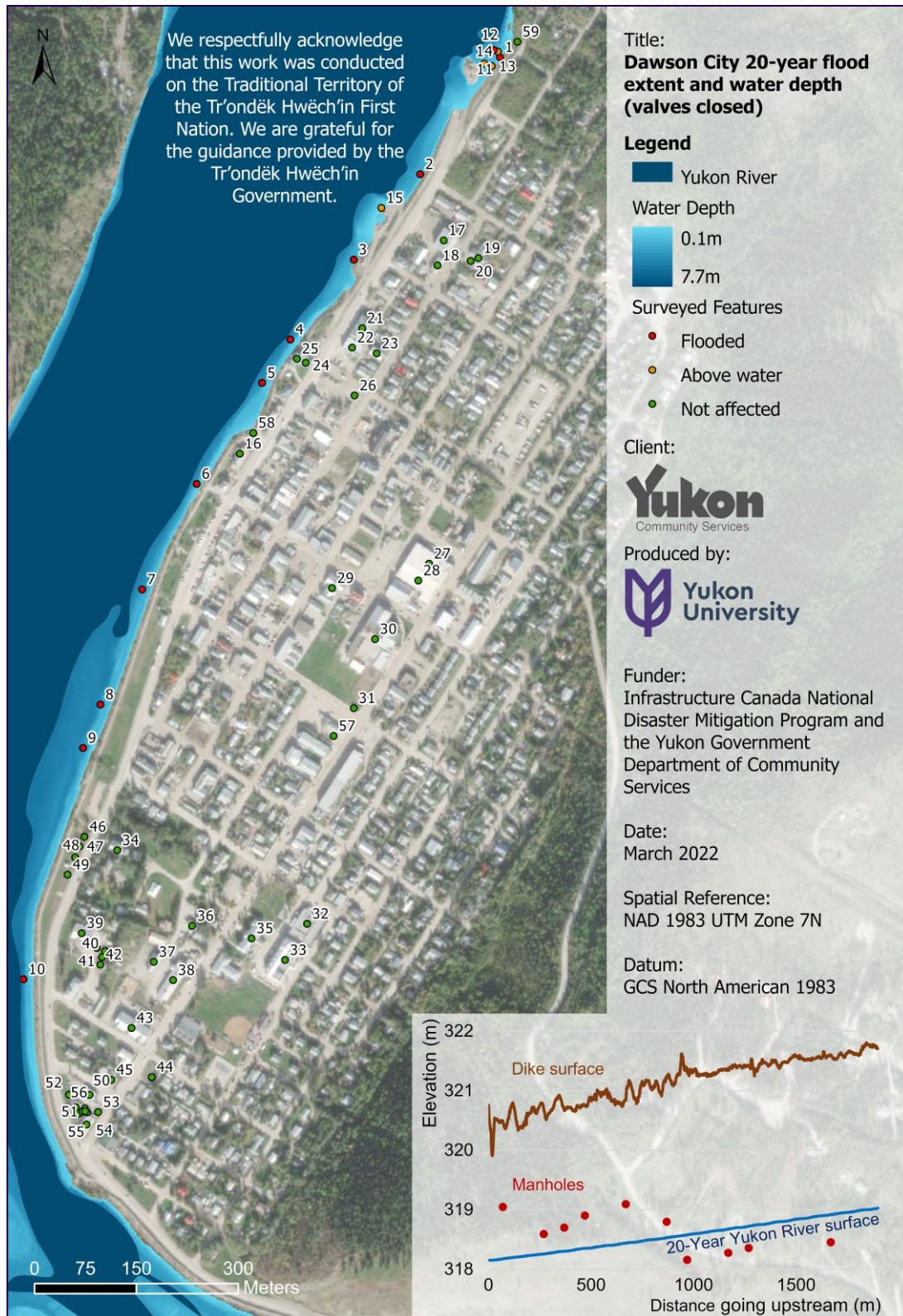
FIGURE 4.2.3. 20-YEAR FLOOD EXTENT (WITH STORM DRAIN VALVES OR MANHOLES CLOSED), WATER DEPTH, AND SURVEYED ASSETS CATEGORIZED BY FLOOD EXPOSURE. NO FLOOD DAMAGE TO REPORT.
